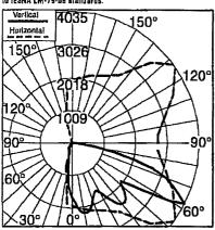
Independent Testing Laboratories certified test. Report No. ITL60824. Candlepower distribution curve of 6 light bar Type IV LEO luminaire with backlight control and 7,080 initial delivered lumens operating at 350mA. All published tumbazire photometric testing performed to LESNA LM-79-BB standards.
