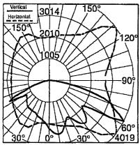
Independent Testing Laboratories certified test. Report No. ITL60829. Candispower distribution curve of 6 light has Type IV LED luminaire with 9,720 initial delivered lumens operating at 350mA. All published luminaire photometric testing performed to ISSNA KM-79-08 standards.
