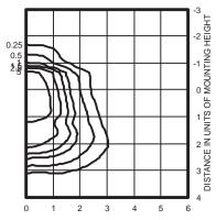
400W pulse start metal halide lamp, rated 38,000 lumens. Footcandle values based on 20' mounting height.
