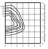
400W pulse start metal halide lamp, rated 42,000 lumens. Footcandle values based on 20' mounting height.
