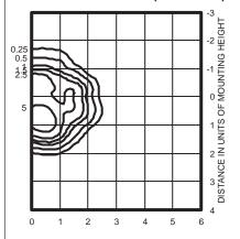
250W pulse start metal halide lamp, rated 22000 lumens. Footcandle values based on 20' mounting height.
