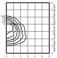
400W pulse start metal halide lamp, rated 38,000 lumens. Footcandle values based on 20'
