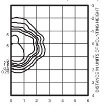
400W pulse start metal halide lamp, rated 36000 lumens. Footcandle values based on 20' mounting height.
