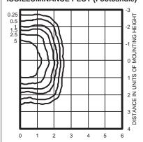
400W pulse start metal halide lamp, rated 38000 lumens. Footcandle values based on 201 mounting height.
