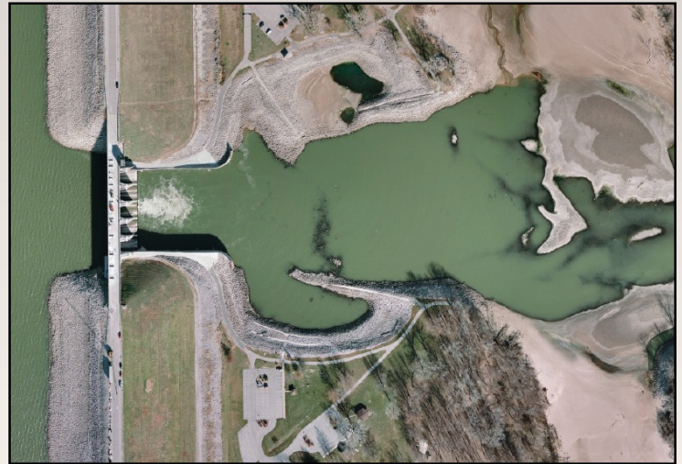
This aerial photograph, which shows the project area at Red Rock Lake and Dam and the Missouri River, was used to generate topographic mapping.
