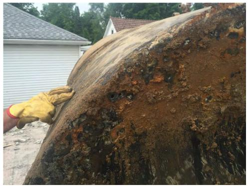
Photograph 7: View of representative view of holes in heating oil UST.
