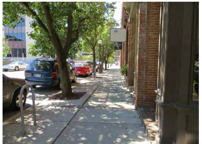
Bike racks and street trees within the Amenity Zone, buffering the pedestrian from the roadway
