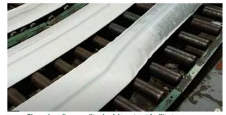
Pipenology liner quality check in wet-out facility to ensure durability and quality.
