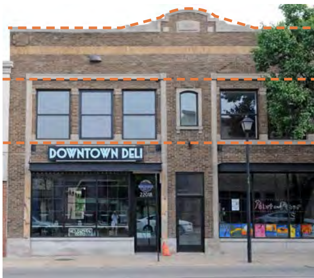
Expression lines create a vertical articulation of base, middle, and top of a facade
