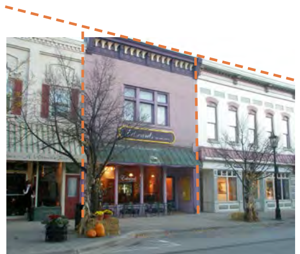
Buildings are organized into horizontally repeated modules to reflect traditional building and lot widths
